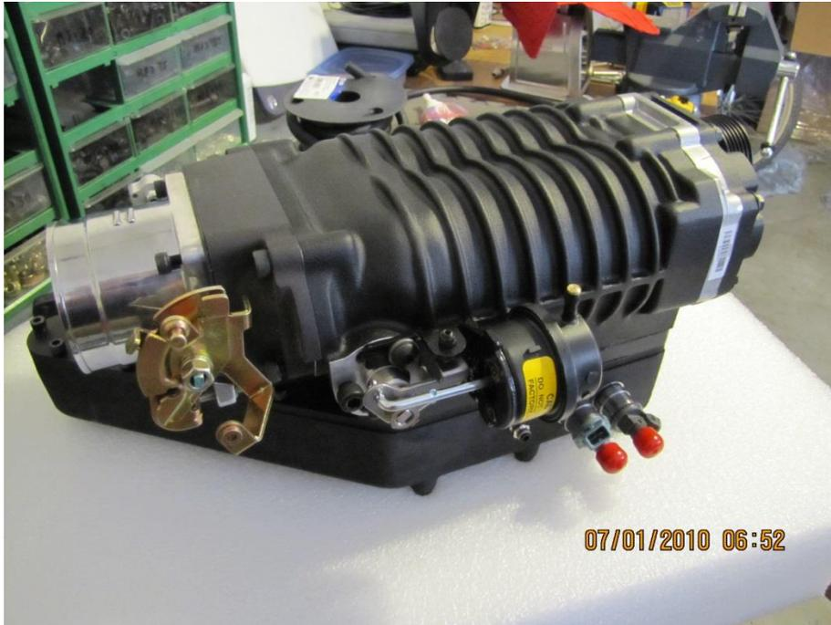
K. The change in direction of the bypass valve also changes the direction of the Throttle Cable Bracket. Note also the parts stack up for the cable pulley on the bracket. The cable then runs around the pulley and back to the crank arm on the TB. Similar to how its mounted stock.
